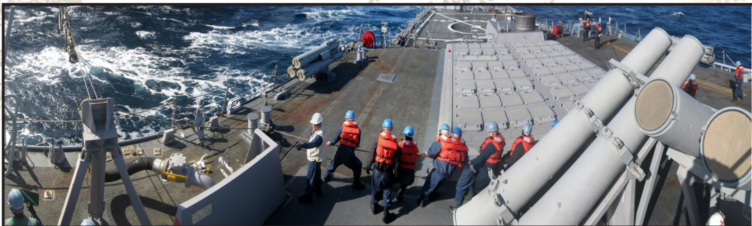
The crew receiving a refueling line from an oil tanker. The Benfold participates in many replenishments while at sea. During this time they receive fuel, mail and other supplies the ship might need. Also in view of this photo are the Tomahawk and Harpoon missiles launchers.
